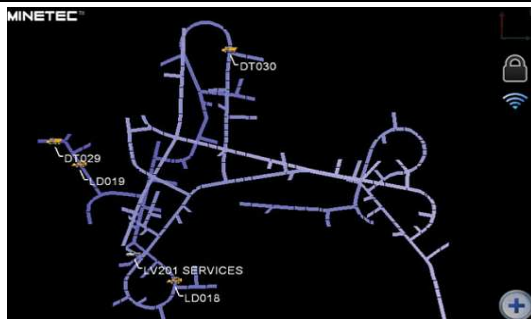
Figure 9: Minetec's Underground Tracking Technology
